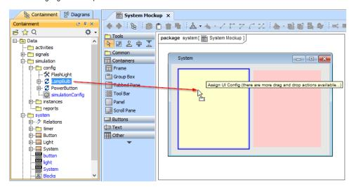
After assigning the LampBulb UI Configuration to the UI panel representing the Light Property, you will see the tagged value Specification of the UI panel that represents the Light property in the Specification of the UI Panel dialog as follows
