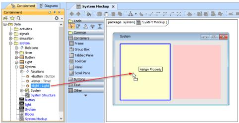
6. Drag an existing UI Configuration named LampBulb to the UI panel that represents the Light property. This will set the dragged UI Configuration to the Config tag of that UI panel as follows
