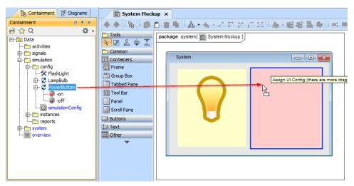
Create a new Simulation Configuration element on any Simulation Configuration diagrams; set the simulationTarget tag to Class system and set the UI tag to the UI Frame that represents the Class system.
