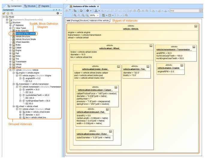
The Block Definition Diagram with instances of the vehicle Block is created by using the Automatic Instantiation wizard. **Sample model**
