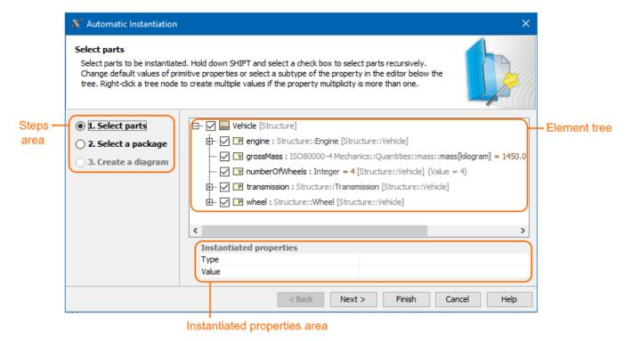
The Automatic Instantiation wizard of the Vehicle Block with highlighted three main areas: Steps area, Element tree, and Instantiated properties area.
