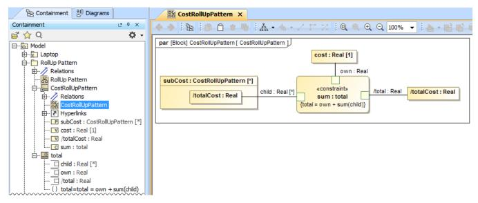
The SysML Parametric Diagram of Cost Rollup Pattern.
