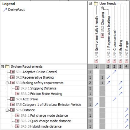
Refine Requirement Matrix allows you to analyze, create, and modify Refine relationships between Requirements and other design
