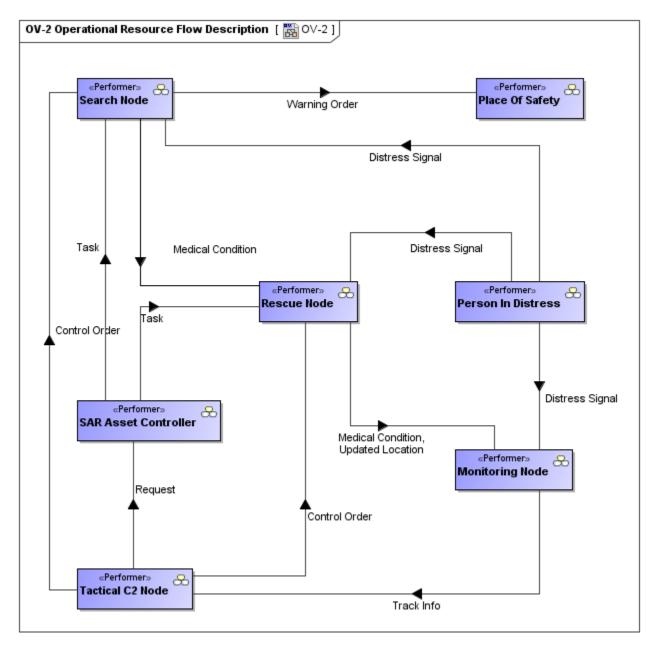
The Needlines established in an OV-2 can be realized by resources and their interactions in a SV-1 Systems Interface Description model or SvcV-1 Services Context Description model.
