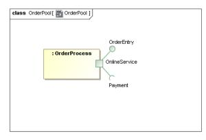
Lollipop and fork symbols in the Composite Structure diagram are implemented as small attachments to a Port symbol similar to name a label. It is not the same as the independent stand alone notation of the interface, it is only part of the port symbol. It is important for Composite Structure diagrams in which real Interfaces (as Classifiers) cannot be used. It is an optional notation as a port does not display provided or required interfaces by default.
