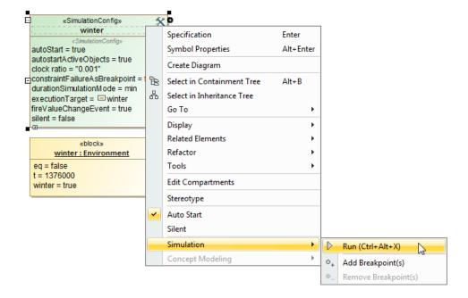
Right-clicking the «SimulationConfig» on the diagram pane to select the Simulation menu to run the simulation of the «SimulationConfig».
