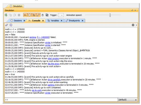
The Console tab in the Simulation window contains the simulation of Activity duration of the DurationConstraint.mdzip sample from start to finish.
