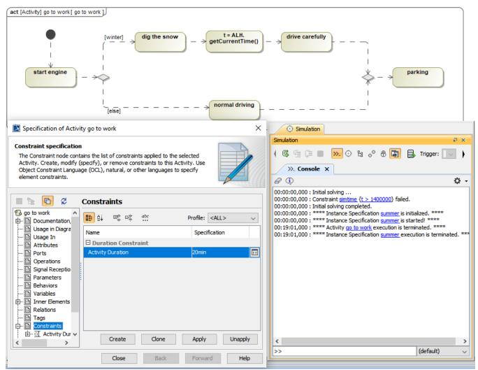
A duration constraint is applied on the Activity as shown on the Console pane.
