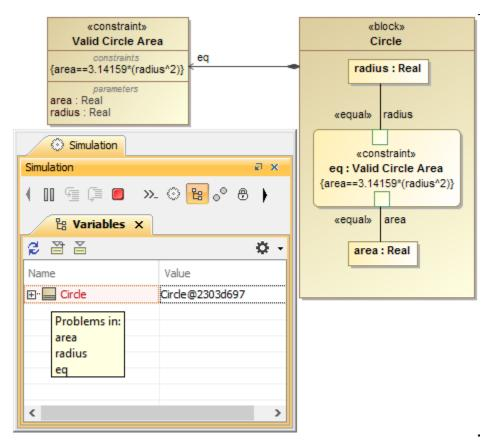
The parent node with a red background indicates failures deeper in the structure tree.
