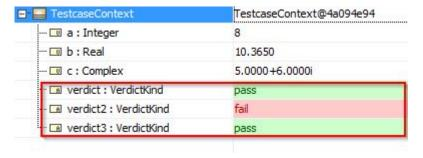
Simulation console showing constraints that have been evaluated.
