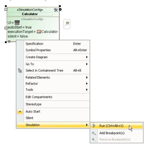
To run a Simulation Configuration through the Simulation Control toolbar
