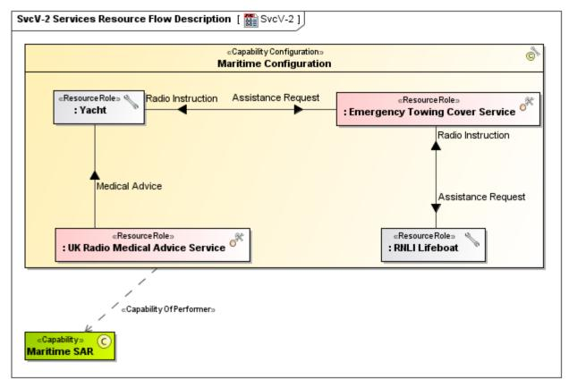
Any protocol referred to in a SvcV-2 diagram needs be defined in the StdV-1 Standards Profile.
