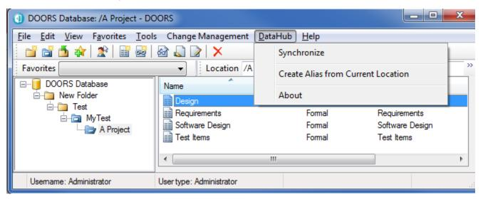
The DataHub menu in the DOORS client main menu provides the functions that you can perform with DataHub as shown in the table below.
