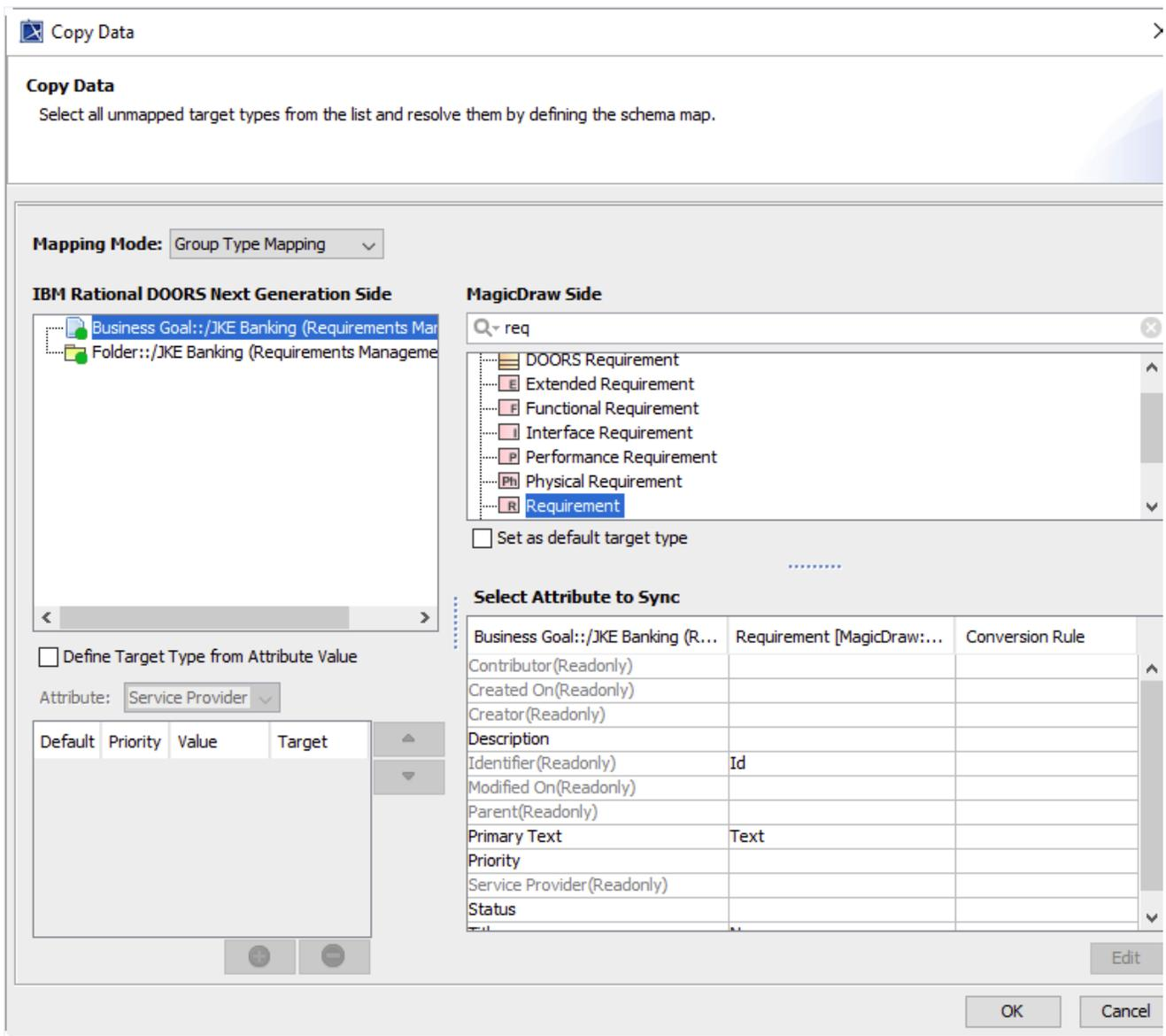
3. Start mapping the source node attributes to target attribute types. You see the node color changing from a red circle to a green one, which means the node and its attributes have been mapped to a target type. The **OK** button becomes enabled at this point. Click **OK** to finish the copying process.
