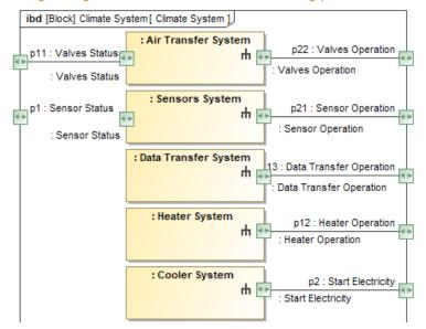
The selected Part Properties in the Climate Control IBD are extracted. As a result the new climate System Block and the SysML Internal Block Diagram are created.
