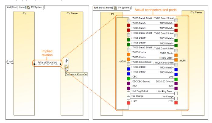
On the left side: the implied relation shows that 18 connectors exist between TV and TV Tuner parts. On the right side: all 18 actual connectors and ports are shown by using the Semantic Zoom In, or Display Underlying Connectors command.
