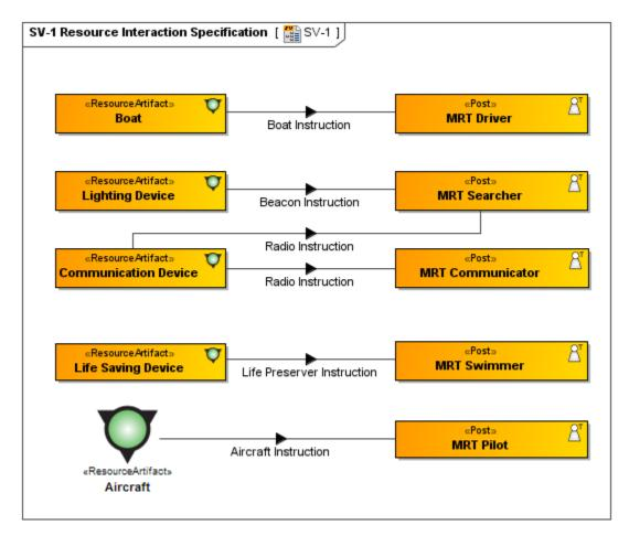
An SV-1 can optionally be adorned with performers originally specified in an OV-2. In this way, traceability can be established from the logical OV structure to the physical SV structure.
