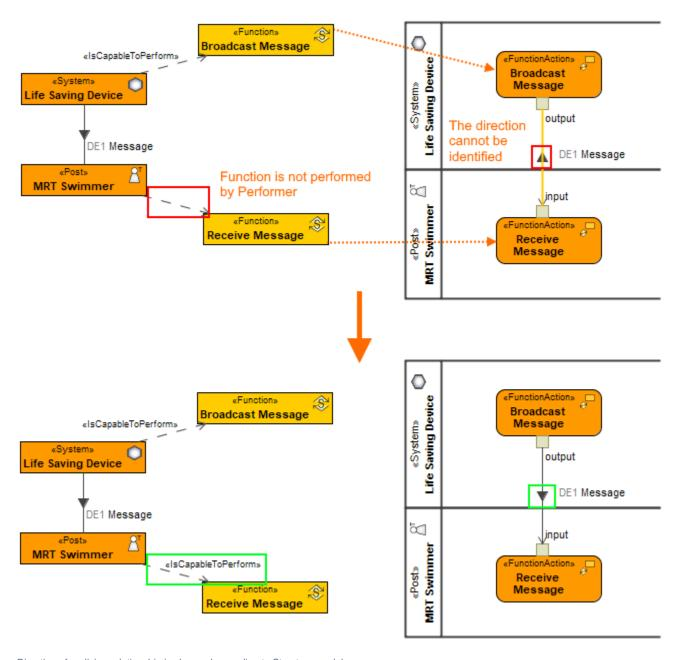
Direction of realizing relationship is changed according to Structure model
