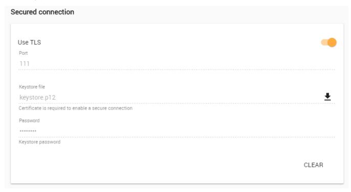
Enabling TLS protocol in TWCloud (when the option is turned on, the color changes to orange).
