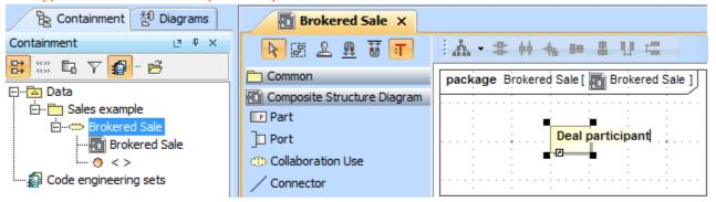
The type for part is created. Typed name on the part = the name of the type.
