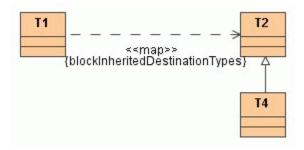
In this case, type T4 has no special treatment. If the user applies the transformation, T1 is mapped to T2. Afterwards the user refines the destination model, changing the attribute type from T2 to T4. If the user now updates the transformation, the attribute type is overwritten: T4 is reset back to T2.
