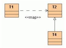
Here T1 is a type in the source domain, while T2 and T4 are types in the destination domain. Given this mapping (T1 > T2), on the first application of the transformation, type T1 residing in the source model will be mapped to type T2 in the destination model.
