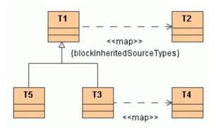
In this case, T3, along with the types derived from it, are still mapped to T4. T1 is still mapped to T2. However, unlike the previous example, T5 and all the types inherited from T1 are NOT mapped to T2.
