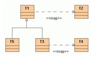
Here T1, T2, and T5 are types in the source domain, while T2 and T4 are types in the destination domain. Given these two mappings (T1 > T2 and T3 > T4), the following statement is true: T1, and all types derived from it (such as T5), are mapped to the T2 type, except T3 and any of the types derived from it. These types are
