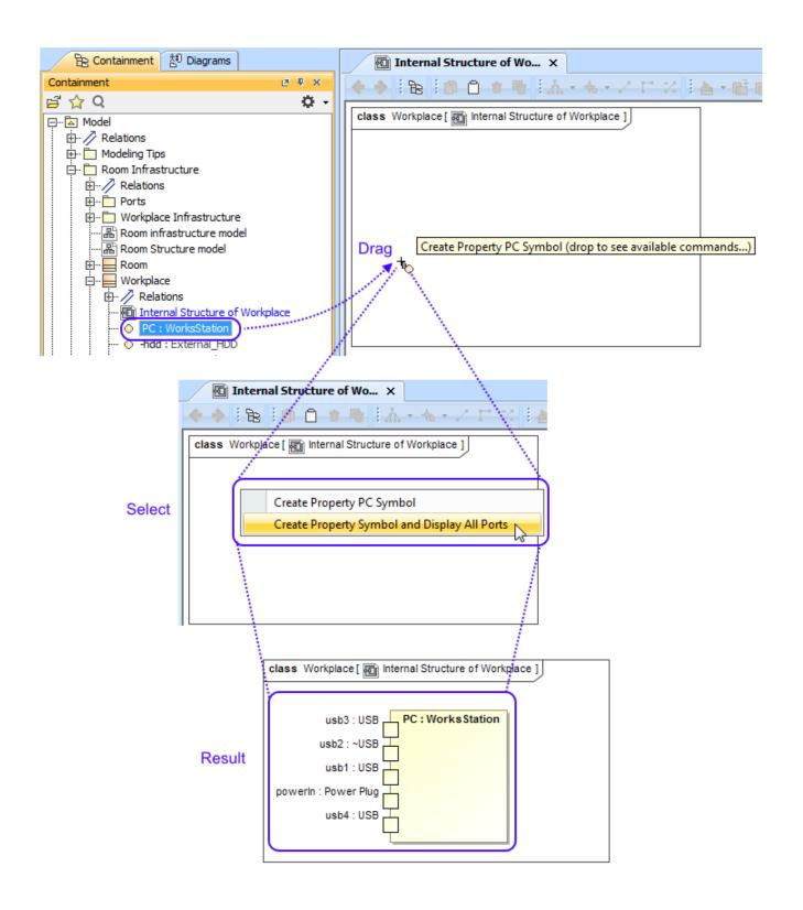
After completing the steps outlined above, the Property shape and/or all its Ports are displayed on the Composite Structure diagram.
