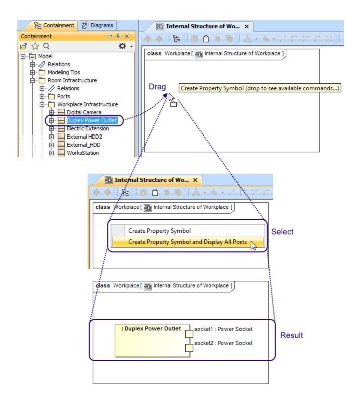
You can display a Property shape by dragging a Property element from the Model Browser to the Composite Structure diagram pane. If this property has P orts defined, you can display them by using the long drag, and selecting an appropriate option from the opened menu (see Example 4).
