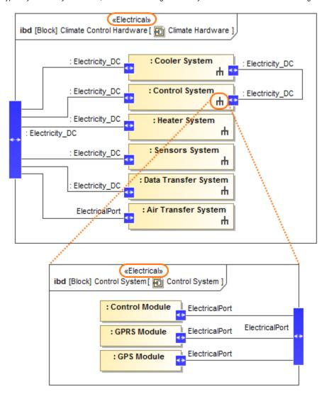
The navigation among aspect diagrams via rake icon. The illustration displays concepts from SysML Plugin.
