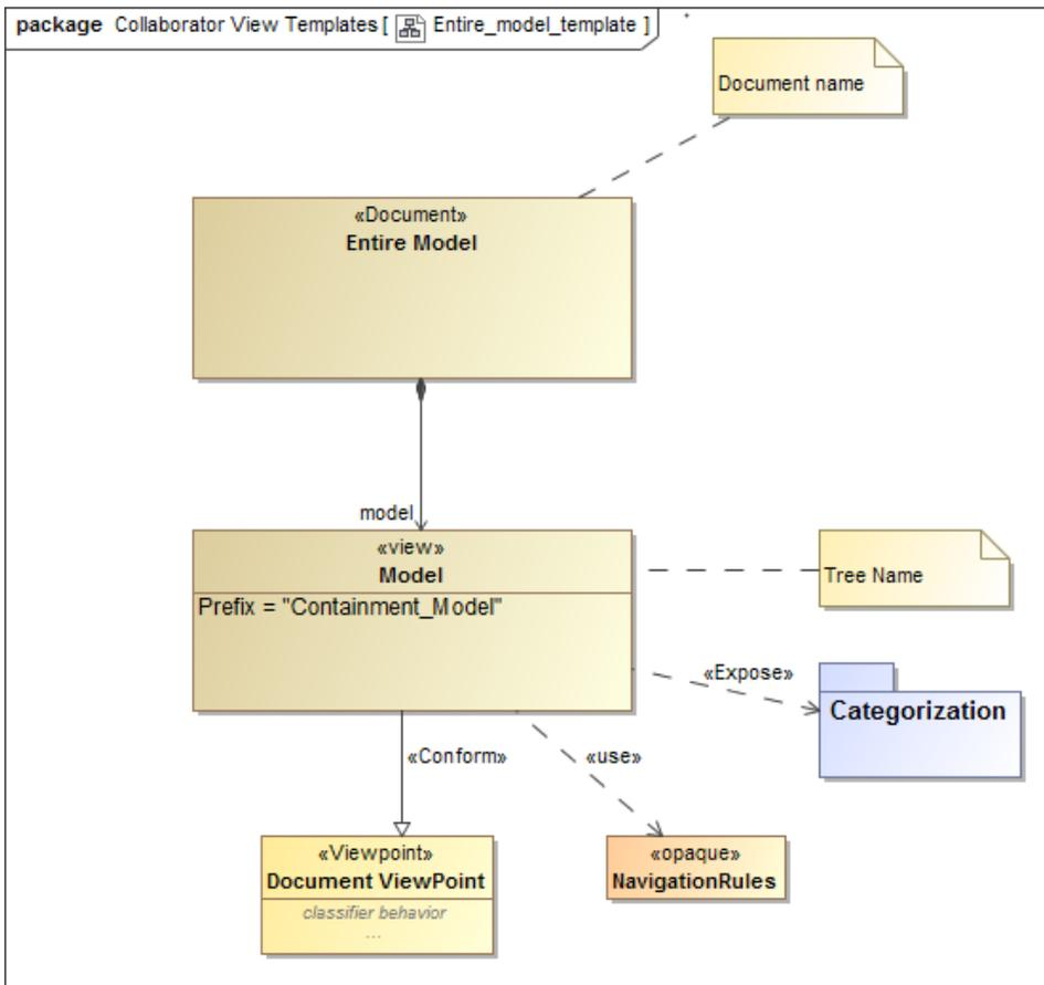
The figure displays the View Diagram of the *Entire Model* template with a default scope that is specified through the «Expose» dependency.
