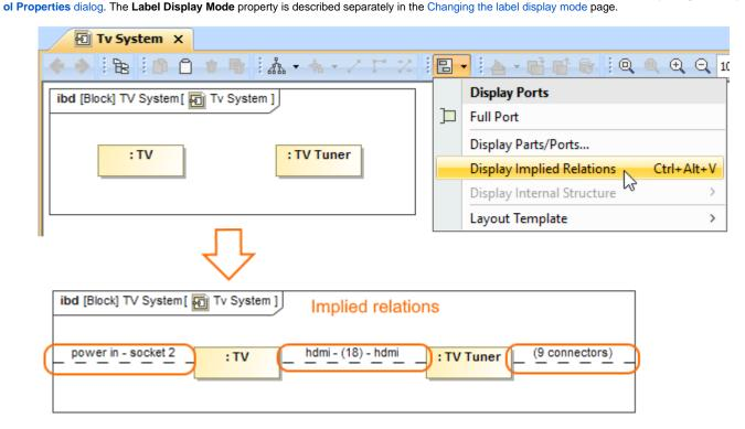
Three implied relations displayed between Part Properties typed by TV and TV Tuner Blocks and diagram frame by using the Display button from the diagram toolbar.
