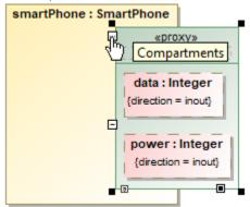
3. Click the Compartments smart manipulator to open the list of properties and select properties you want to display in the Port shape.
