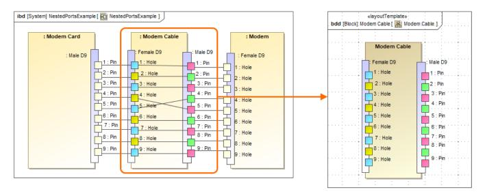
Creating a layout template from the SysML Internal Block Diagram (Composite Structure Diagram in a UML project).
