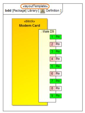
The Definition BDD is set as the layout template named Definition. The illustration displays concepts from SysML Plugin.
