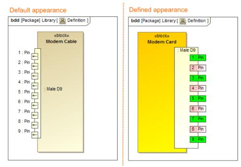
The comparison of default and defined appearance of the Modem Card Block, style, and the position of its ports. The illustration displays concepts from SysML Plugin.
