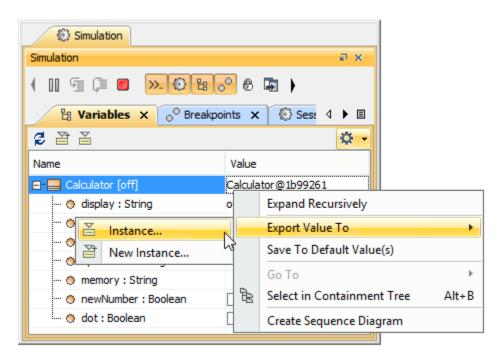
export the value of a runtime object using this method, the runtime object must be created from a Classifier.
