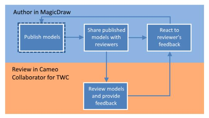
Publishing a model is the first step in the workflow for reviewing models and providing feedback.
