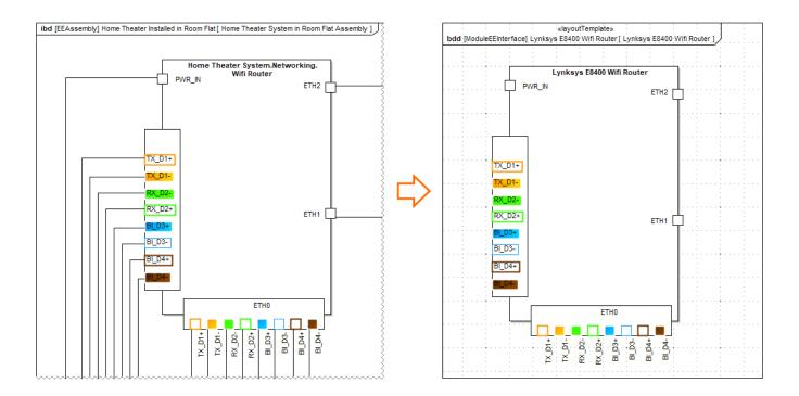
Layout template created from the Internal Block Diagram.
