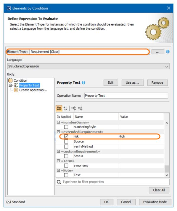
The Elements by Condition dialog with the Property Test operation defined to test if Requirements have a high risk level.
