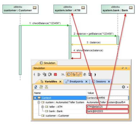
Simulation console showing how a lifeline with a dot notation can represent a nested property.
