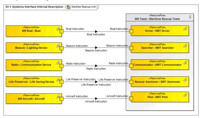
An SV-1 can optionally be adorned with performers originally specified in an OV-2. In this way, traceability can be established from the logical OV structure to the physical SV structure.
