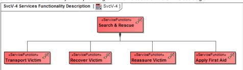
SvcV-4 Services Functionality Flow Description diagram which is based on the UML Activity diagram.
