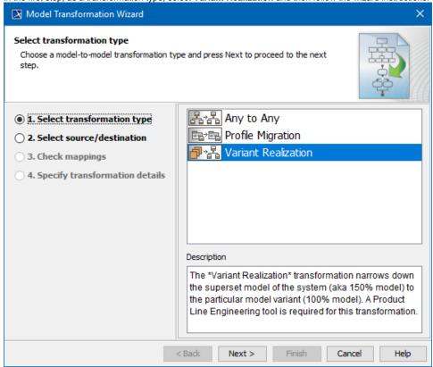
6. in the last step, Specify transformation details, you can clean variation point data after transformation. If you set this property to true, all the variation points applied on a transformed element are removed from the resultant model.
