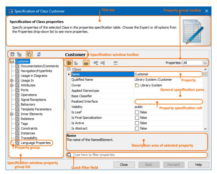
The Specification window is used to define UML model elements such as class, package, activity. The Specification window is a non-modal window in which you can edit model element property values and work with a model simultaneously.
