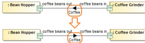
The direction of *Coffee* Information Flow is reversed. The illustration displays concepts from SysML Plugin.
