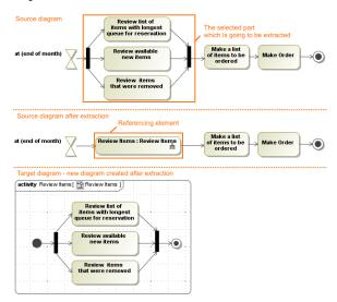
As you can see in the example, during extraction, the selected part of the activity diagram is moved to the newly created *Review Items* activity diagram. In the source diagram, a *Review Items* call behavior action is created in place of the selected elements.
