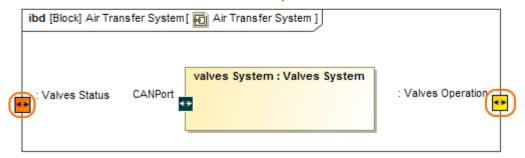
The layout template applied on the Air Transfer System Internal Block Diagram frame.
