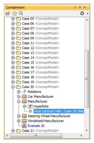
The Concept Modeler highlights the subsetted property in the Containment tree.
