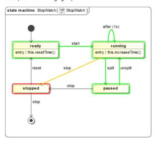
In the *stopped* state, if the *reset* Signal is sent to the *StopWatch* object, the object will go to the *ready* State, and the *time* value will be reset to zero by calling the *resetTime* operation. If, instead, the *stop* Signal is sent to the object again, the object will go to the Final State, the simulation will stop, and all of the simulation sessions will be closed.
