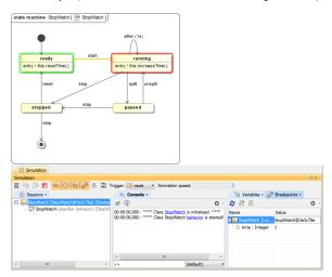
The *StopWatch* object stays in the *running* State, and the Time Event is triggered in this State every second. Therefore, a new simulation session will be created to call the *increaseTime* operation every second, and the *time* value will increment by one every time the operation is executed (see the following figure).
