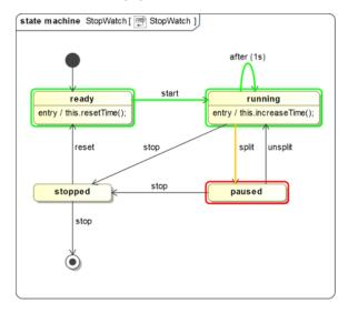
You can transition the paused *StopWatch* object to the *running* state by sending an *unsplit* Signal to the object.
