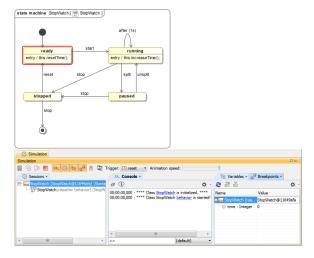
Now we want to trigger the *StopWatch* object to move from the *ready* State to the *running* State. To do this, we need to send a *start* signal to the *StopWatch* object.
