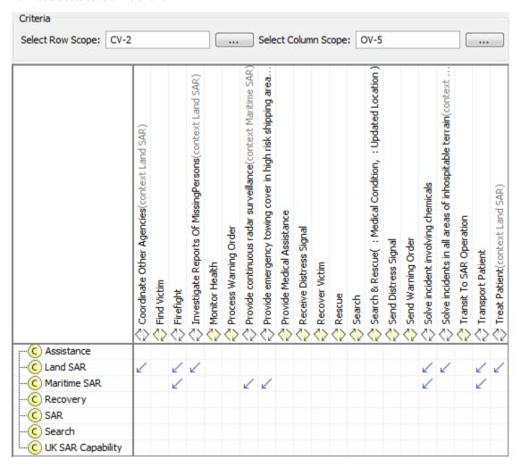
This model is analogous to the SV-5a Operational Activity to System Function Traceability Matrix – but provides the interface between Capability and Operational Models rather than Operational to System Models.
