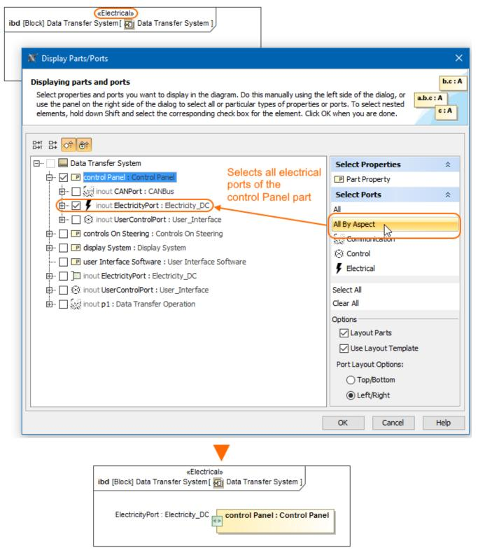
The All By Aspect button usage in the Display Parts/Ports dialog. The illustration displays concepts from SysML Plugin.
