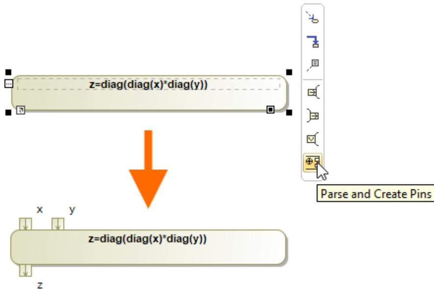
On top border of the Opaque Action, the input pins x and y are created, and on the bottom border, the output pin is created.
