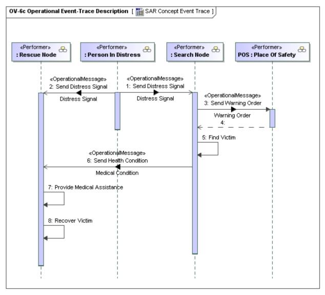
The information content of messages in an OV-6c may be related with the Resource Flows in the OV-3 Operational Resource Flow Matrix and OV-5b Operational Activity Model and information entities in the DIV-2 Logical Data Model.
