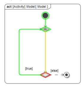
The model runs an infinite loop until StackOverflowError occurs, and the execution is terminated.
