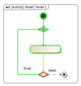
The model runs an infinite loop without StackOverflowError, and the execution is not terminated.
