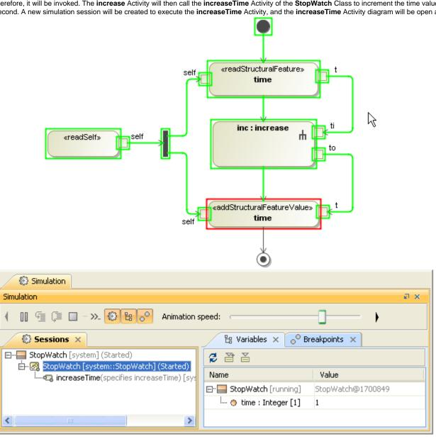
The increaseTime Activity will be completely executed when its Final stage has been reached. Once the execution is complete, the simulation session of the increaseTime Activity will be closed and the StopWatch State Machine will be activated again. Now you can see in the Variables tab that the time value of the StopWatch object has been incremented by one.
