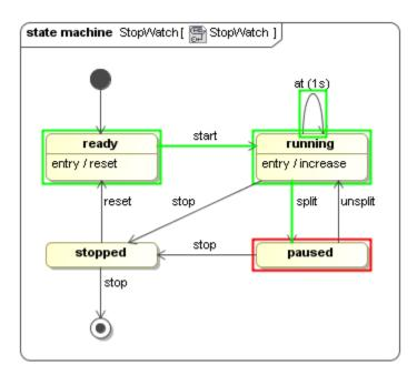
You can change the paused StopWatch object to the running State by sending an unsplit signal to the object.
