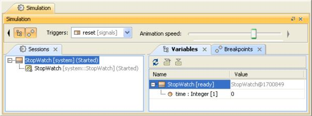
Now we want to trigger the StopWatch object from the ready State to the running State. To do this, we need to send a start signal to the StopWatch object.
