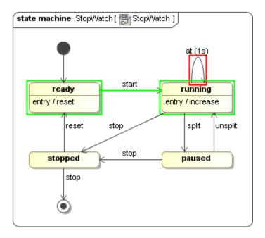
While the StopWatch object is at the **running** State, we can send a **split** signal to trigger the object to the **paused** State or send a **stop** signal to trigger the object to the **stopped** State.
