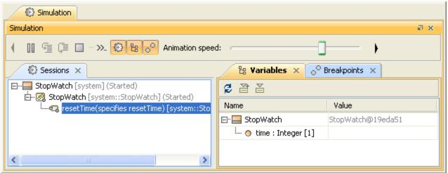
The execution of the **resetTime** Activity will be terminated once it has reached the final stage. When the simulation stops, the session executing the **resetTi me** Activity will be closed, the StopWatch State Machine diagram will be reactivated, and the simulation will wait for an Event signal at the ready State. You can browse the **StopWatch** object in the **Variables** tab to see the time value.
