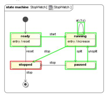
At the **stopped** State, if the **reset** signal is sent to the StopWatch object, the object will go to the **ready** State, and the time value will be reset to zero at the entry to the **ready** state by calling the **resetTime** Activity. If the **stop** signal is sent to the object again, the object will go to the final stage, and then the simulation will stop and all of the simulation sessions will be closed.
