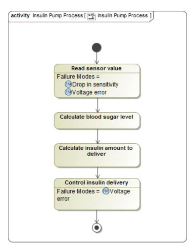
In this Activity Diagram, the Read sensor value and Control insulin delivery Actions are linked to the Drop in sensitivity and Voltage error Failure Modes.
