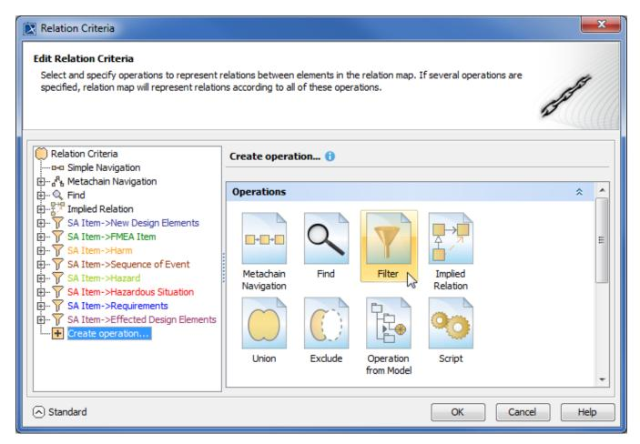
In the Expert mode, the Relation Criteria dialog allows you to create a new Filter operation, and define it to represent a desired relation.
